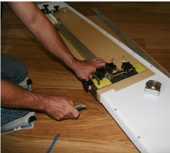
Treadman®'s adjusted edges, ready for cutting
