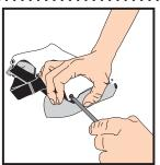
Reattach Rubber Boot with screws.
