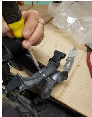
5. Remove Strap Mount screws.
