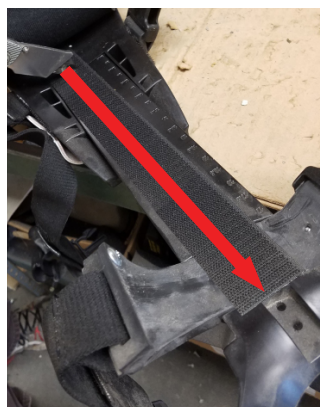
7. Cut new Hook 'n Loop strip from kneeseat to end of Strap Mount (Note: New Hook 'n Loop strip approx. 1.5" longer than old)
