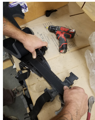
8. Firmly press Hook 'n Loop strip onto frame and over screw heads and then re-secure Cushion with supplied cable tie.
