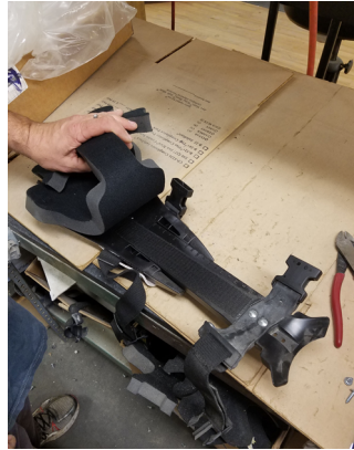
2. Pull back Cushion Insert revealing Strap Mount screws and Hook 'n Loop.
